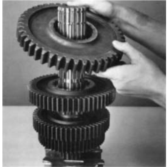
14. Install the LO speed gear on shaft against 1st speed gear, clutching teeth up.
