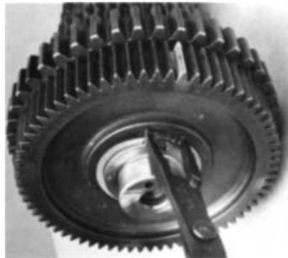
10. Remove each remaining gear, limit washer, spacer and sliding clutch from mainshaft in the same manner previously detailed. And, if necessary, remove the snap ring from I.D. of each gear.
