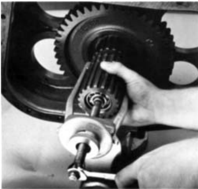
4. Insert jaws of puller behind range mainshaft and pull from quill.
