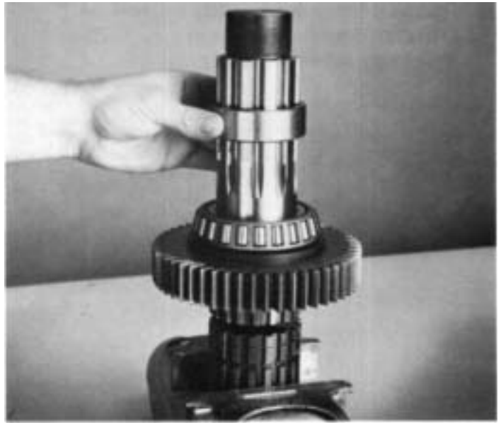
7. Install the bearing inner spacer on output shaft.
