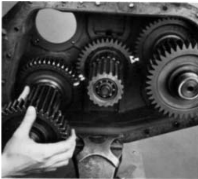
3. Remove both auxiliary countershafts.
