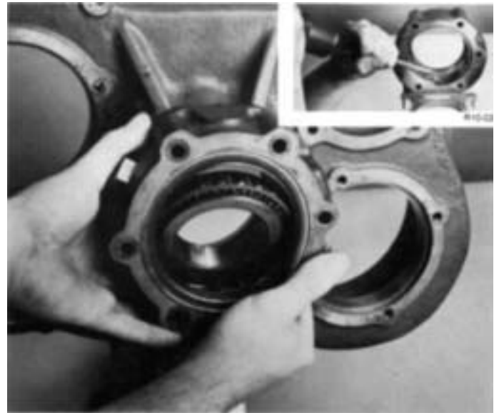
7. Turn out the capscrews and remove the rear bearing cover and gasket. The rear bearing cone will drop from bore in auxiliary plate when cover is removed. If necessary, remove the oil seal from cover (inset).
