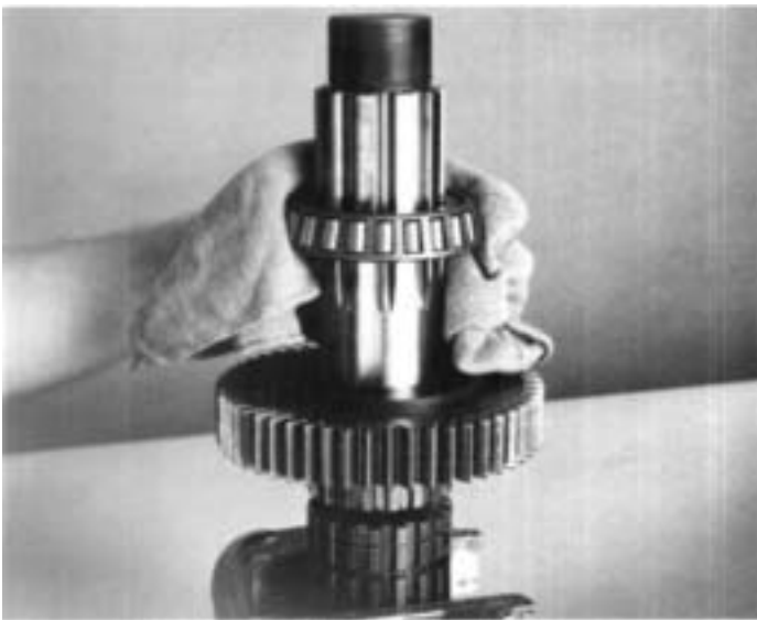
6. Heat the front bearing cone and install on output shaft against washer, bearing taper up. NOTE: DO NOT HEAT BEARING ABOVE 275°F (136°C). If possible, use heat lamps as source.
