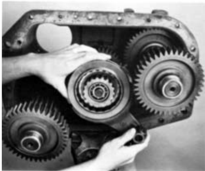
2. Remove splitter shift yoke and sliding clutch.
