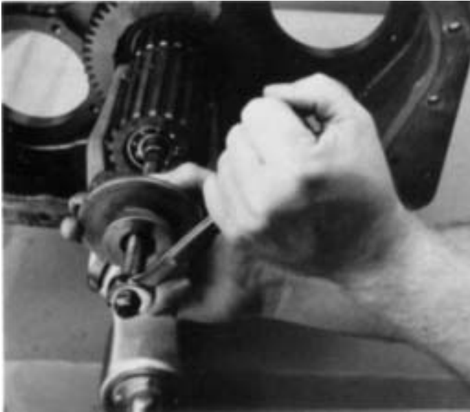
5. Remove range mainshaft with jaw puller.
