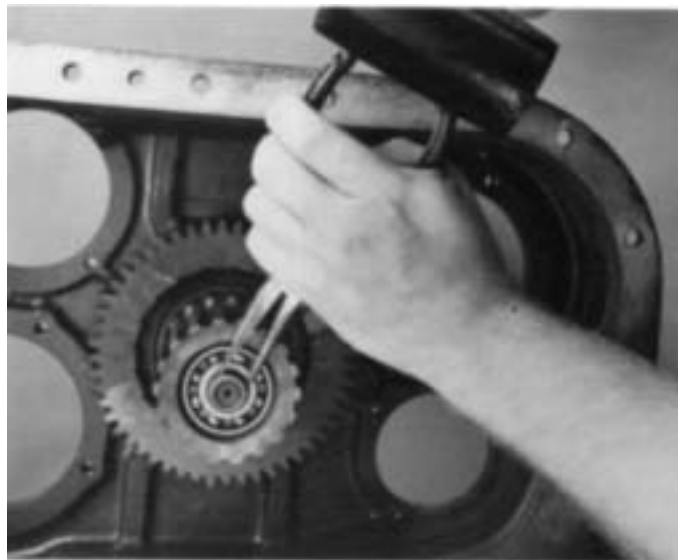
4. Remove the "C" ring from the groove at front of mainshaft quill.
