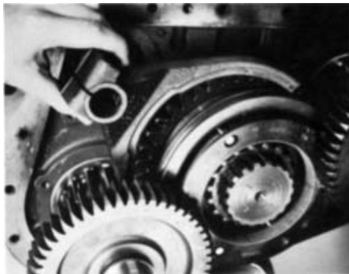
5. Remove range yoke from sliding clutch of synchronizer assembly.
