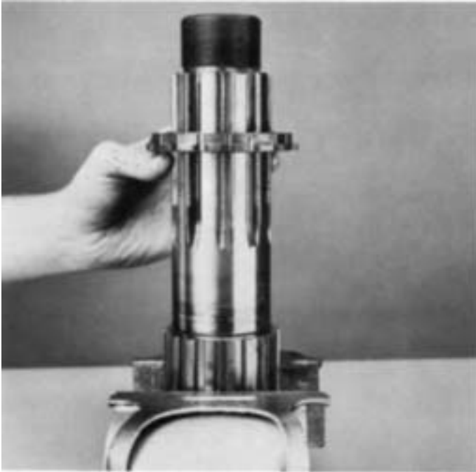
5. Remove the splined spacer from output shaft.
