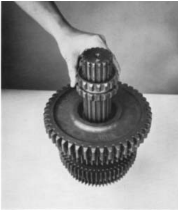
7. Remove the LO-Reverse speed sliding clutch from mainshaft.
