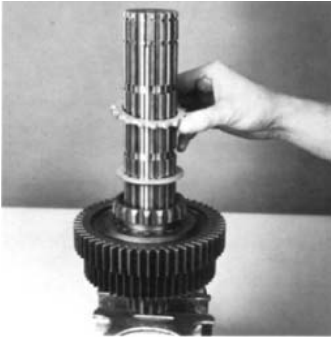
12. Install the spacer on shaft against washer.
