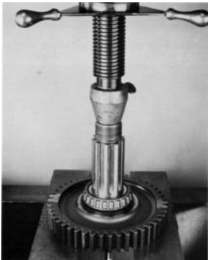
8. Using the front face of deep reduction gear as a base, press the output shaft through the bearing and gear. This will free the bearing, gear, washer, and, for models so equipped, the spacer or oil retention ring. DO NOT DAMAGE MAINSHAFT QUILL.
