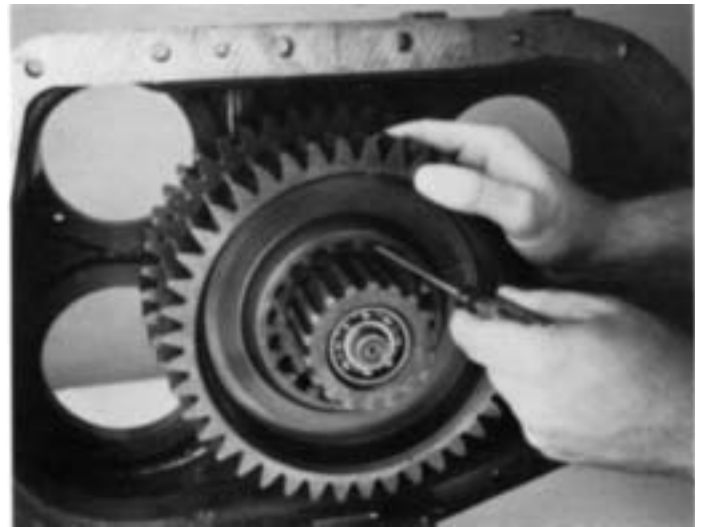
2. Turn the washer located in the hub at low range gear so that the splines of washer align with the splines of mainshaft.
