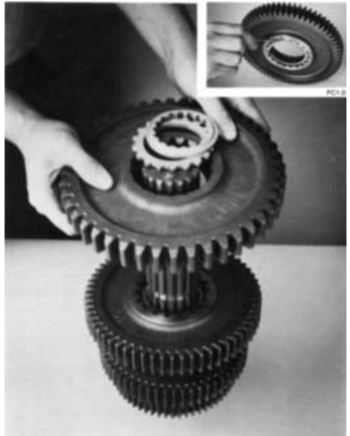
9. Pull the LO speed gear from rear of mainshaft to remove limit washer, spacer and gear. If necessary, remove the snap ring from I.D. of gear (inset).
