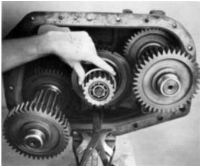
1. Remove the snap ring from the groove of range mainshaft.
