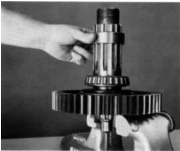
7. Remove the bearing inner spacer from output shaft.
