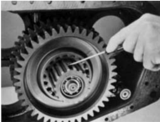
1. Remove the key from keyway of range mainshaft.
