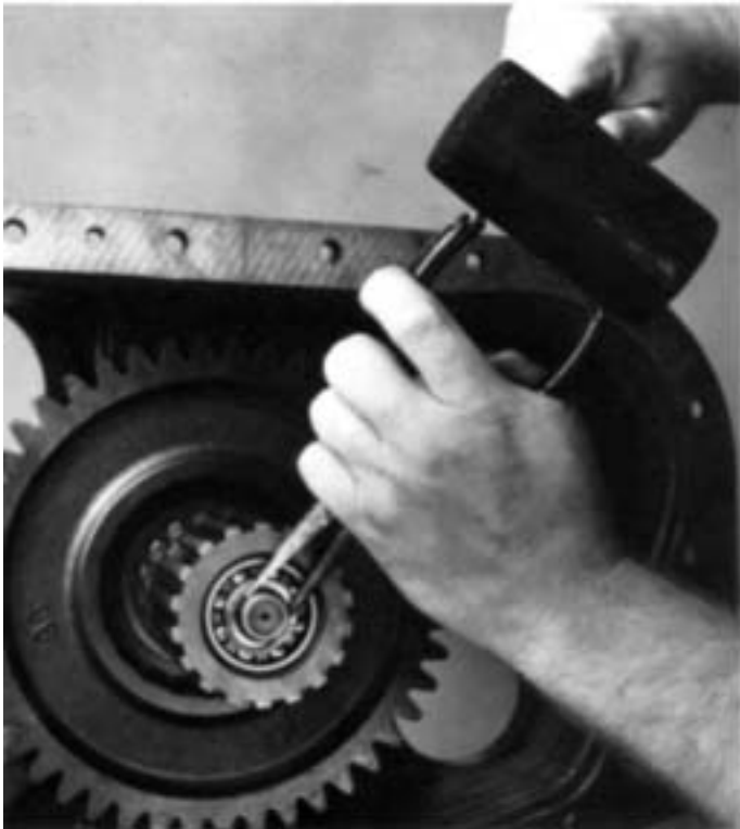
3. Remove the "C" ring from groove at front of mainshaft quill.
