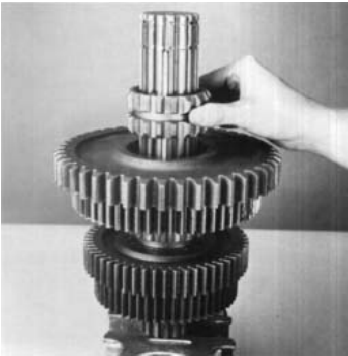
18. Install the LO-Reverse speed sliding clutch, aligning the missing internal spline of sliding clutch with key in mainshaft.
